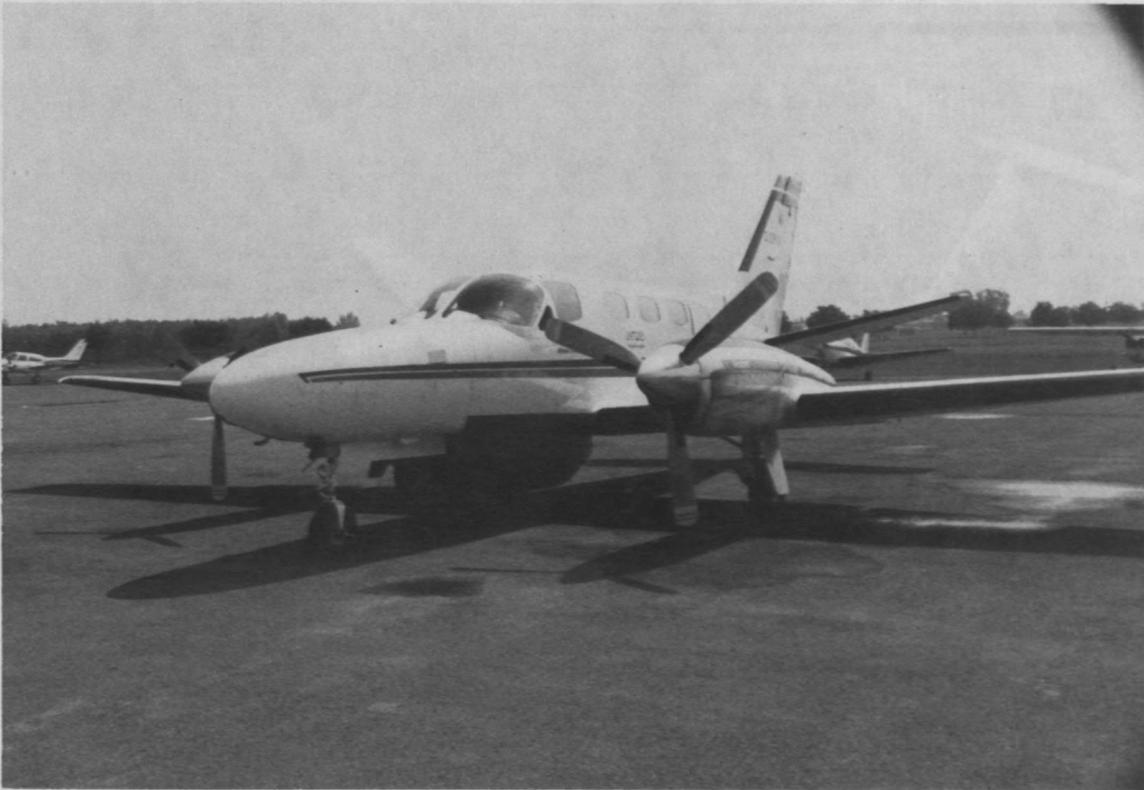
Figure 4. Twin-engine Cessna Conquest equipped with a synthetic aperture radar. The Conquest is a cost-effective platform which delivers the altitude, range and speed capabilities required to operate a SAR. The Conquest provides a service ceiling of about 11,275 metres and has a maximum range of about 4,000 kilometres when flying at 10,000 metres. The aircraft would also make a good platform for an infrared linescanner and/or a camera system. (Courtesy Intera Technologies Ltd.)
