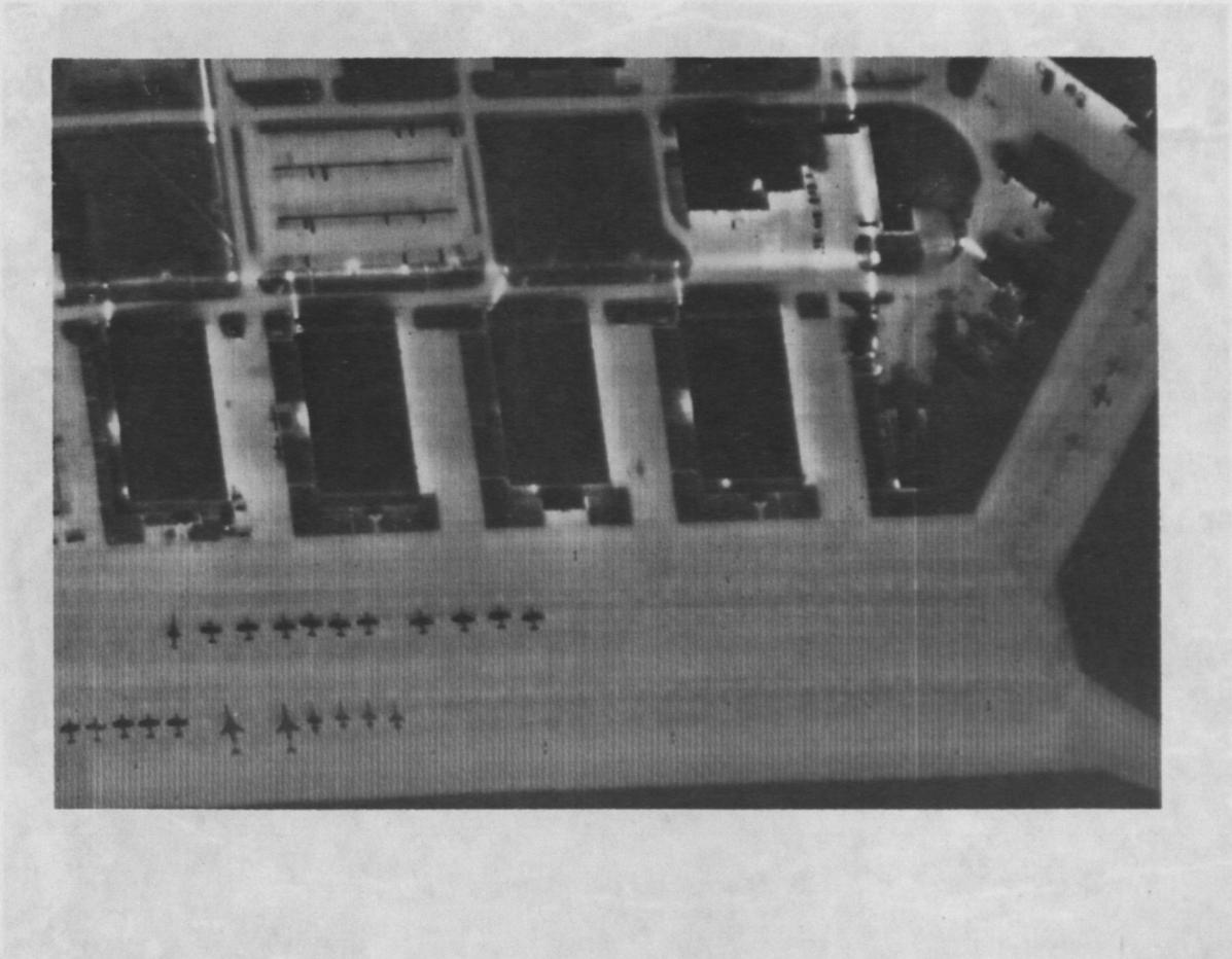
Figure 2. This thermal infrared linescanner image shows the utility of this sensor to map heat sources that are indicative of the level of human activity. Note the buried heating lines and the heat escaping from the hangar doors. The spatial resolution of this image is approximately 50 centimetres and the thermal resolution is 0.2 degrees Celsius.
