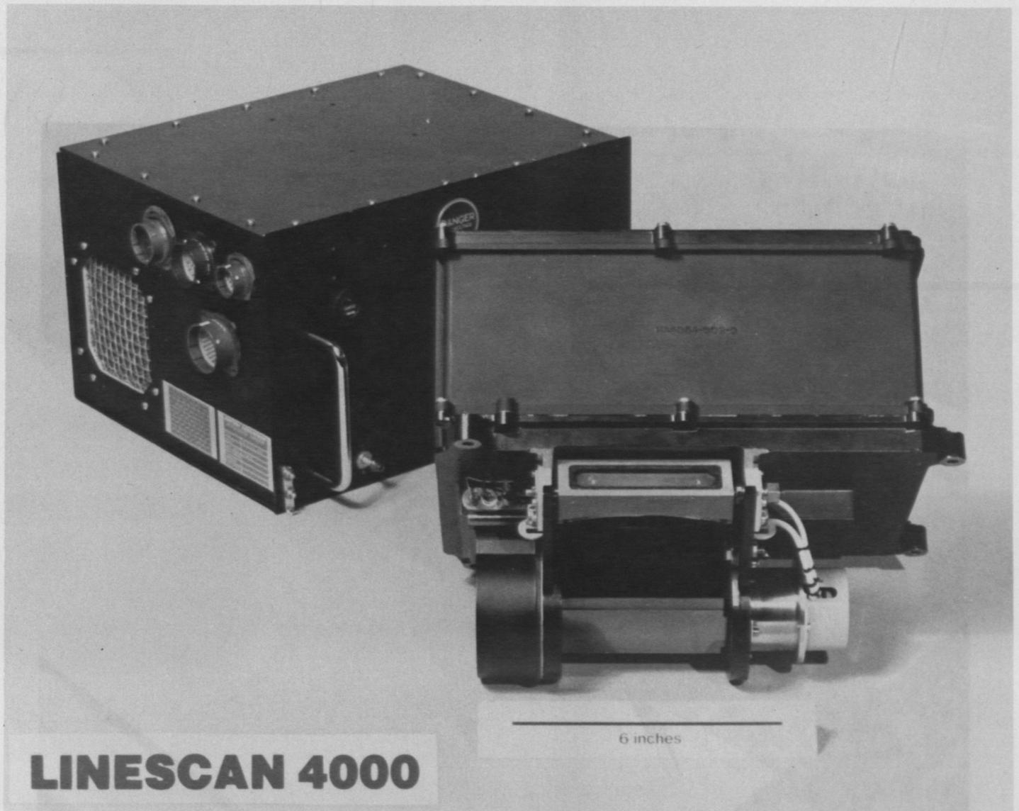
Figure 12. Linescan 4000 infrared linescan system. The system is compact and can be used on a wide range of platforms. It provides horizon-to-horizon coverage, electronic roll stabilization, real time video output and can be down-linked to a ground station. It has a multi-element mercury cadmium telluride detector operating in the 8 to 14  $\mu\text{m}$  waveband and a closed cycle helium detector cooling system. (Courtesy of Vinten Military Systems Ltd.)
