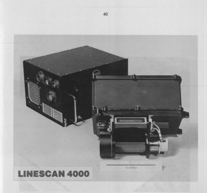
Figure 12. Linescan 4000 infrared linescan system. The system is compact and can be used on a wide range of platforms. It provides horizon-to-horizon coverage, electronic roll stabilization, real time video output and can be down-linked to a ground station. It has a multi-element mercury cadmium telluride detector operating in the 8 to 14  $\mu$ m waveband and a closed cycle helium detector cooling system. (Courtesy of Vinten Military Systems Ltd.)
