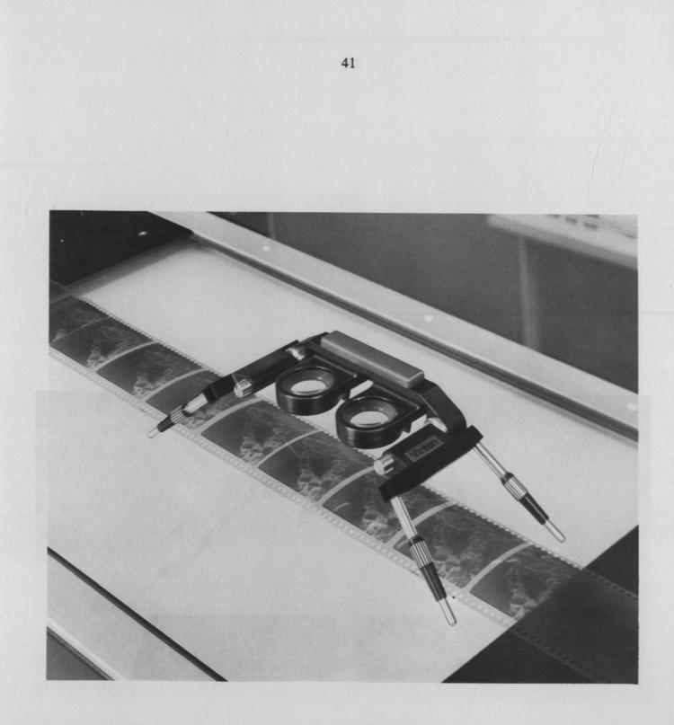
Figure 13. Lens stereoscope with 2x and 4x magnification lenses. (Courtesy of Vinten Military Systems Ltd.)
