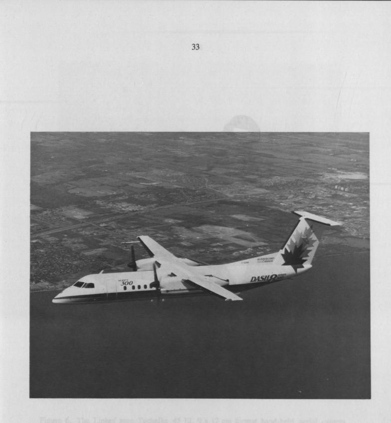
Figure 5. The Boeing Dash 8 Series 300 provides a large volume platform, with room for 16 passengers or more as well as a full complement of sensors. The aircraft could be used to transport on-site inspection teams as well as being a sensor platform. (Courtesy of Boeing Canada, de Havilland Division)
