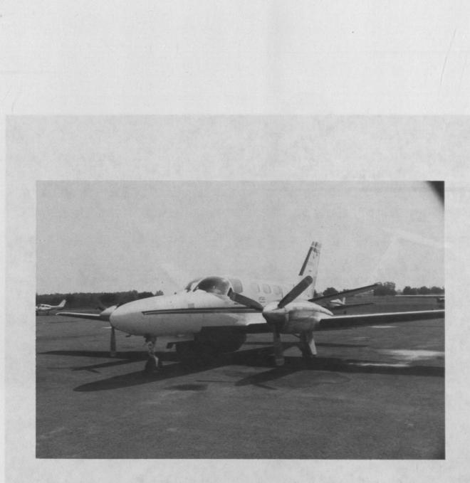
Figure 4. Twin-engined Cessna Conquest equipped with a synthetic aperture radar. The Conquest is a cost-effective platform which delivers the altitude, range and speed capabilities required to operate a SAR. The Conquest provides a service ceiling of about 11,275 metres and has a maximum range of about 4,000 kilometres when flying at 10,000 metres. The aircraft would also make a good platform for an infrared linescanner and/or a camera system. (Courtesy Intera Technologies Ltd.)
