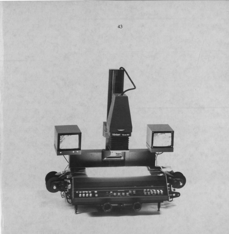
Figure 15. The Vinten Vicon 80 Imagery Interpretation and Reporting System. Based upon a closed circuit television system, the Vicon 80 provides a system for rapid presentation, enhancement and visual interpretation of film-based imagery. (Courtesy of Vinten Military Systems Ltd.)
