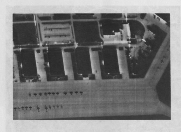
Figure 2. This thermal infrared linescanner image shows the utility of this sensor to map heat sources that are indicative of the level of human activity. Note the buried heating lines and the heat escaping from the hangar doors. The spatial resolution of this image is approximately 50 centimetres and the thermal resolution is 0.2 degrees Celsius.
