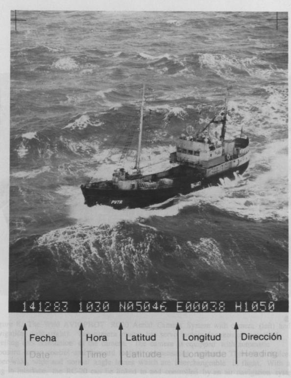
Figure 7. Oblique photograph taken using an Agiflite hand-held camera with time and position data recorded in the margin at the time of exposure. (Courtesy of Negretti Aviation)
