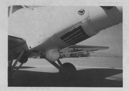
Figure 11. Two Honeywell Gimbaled Mark III FLIR systems mounted fore and aft under the fuselage of an Ayres S2/R Turbo Thrush aircraft. (Courtesy of Dave Dorschner, Aviation Resource Management.)
