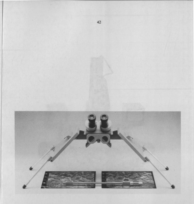
Figure 14. Sokkisha MS27 mirror stereoscope with a pair of aerial photographs prepared for stereo viewing together with a parallax bar. (Courtesy of Mark Lystiuk, Currie Engineering, and Sokkisha Co., Ltd.)
