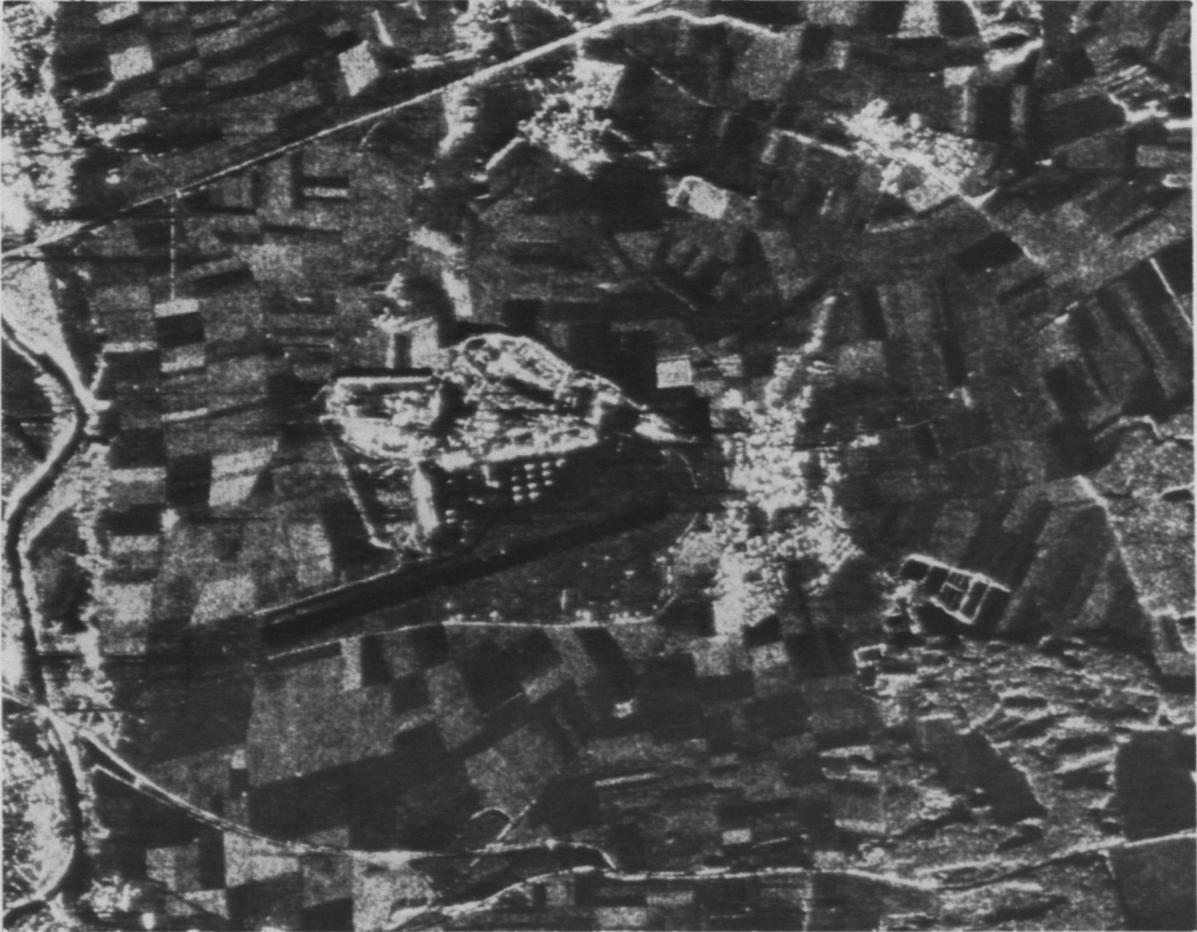
Figure 3. This synthetic aperture radar image was acquired from an altitude of 11,000 metres. Note the broad area coverage provided by SAR and the reflective characteristics of the vehicles, perimeter fence and buildings. The spatial resolution of this image is approximately six metres. (This would also make a good platform for an infrared line scanner and/or a camera system. (Courtesy Inera Technologies Ltd.)
