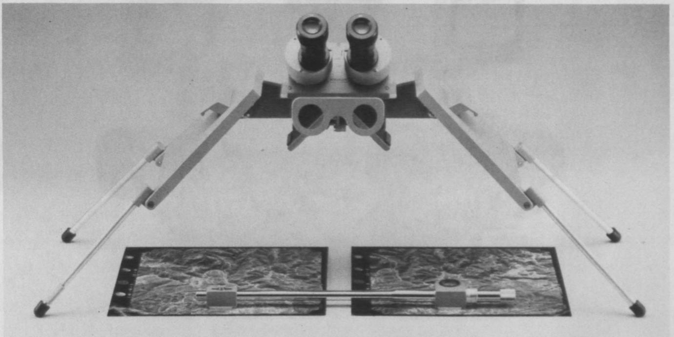
Figure 14. Sokkisha MS27 mirror stereoscope with a pair of aerial photographs prepared for stereo viewing together with a parallax bar. (Courtesy of Mark Lystiuk, Currie Engineering, and Sokkisha Co., Ltd.)
