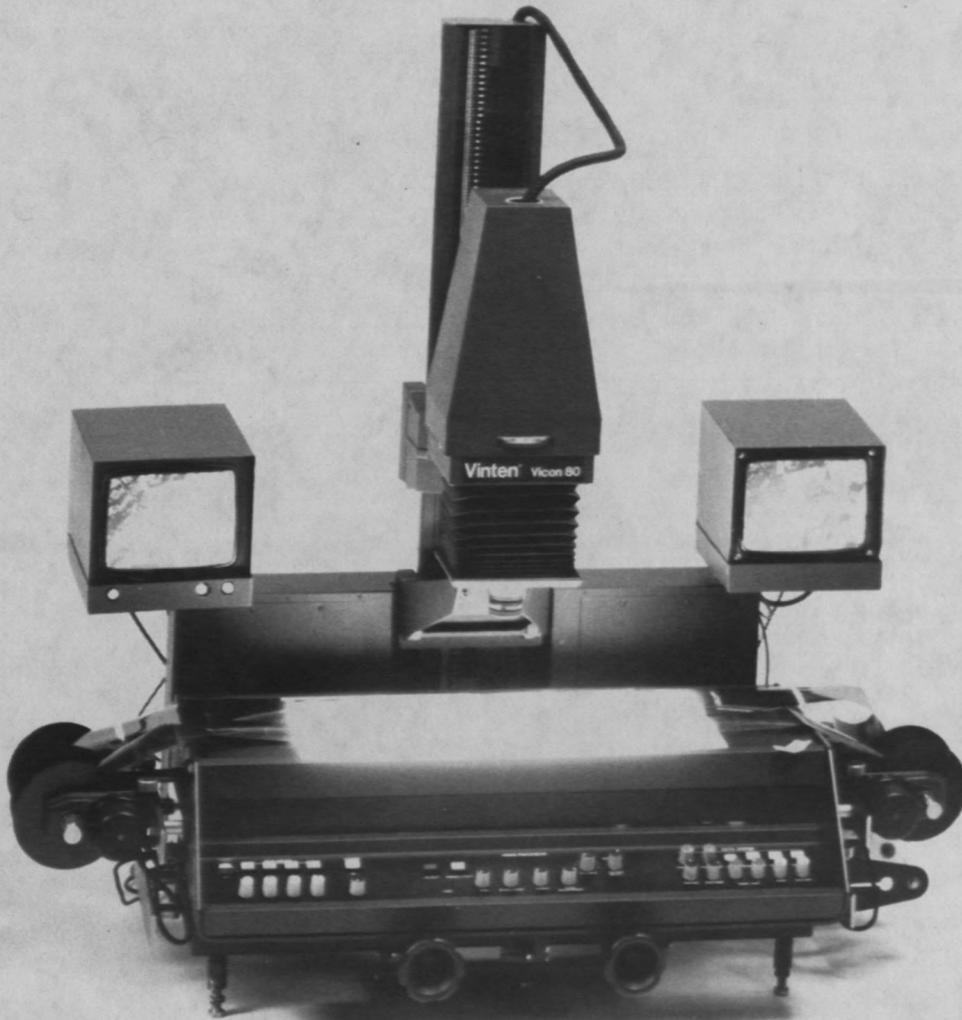
Figure 15. The Vinten Vicon 80 Imagery Interpretation and Reporting System. Based upon a closed circuit television system, the Vicon 80 provides a system for rapid presentation, enhancement and visual interpretation of film-based imagery. (Courtesy of Vinten Military Systems Ltd.)
