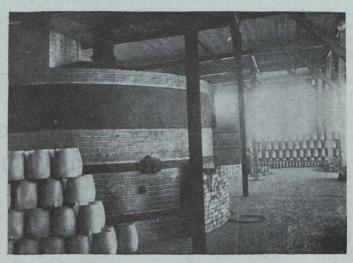
Top of Kilns, which extend from Basement. Firing is done on a lower floor.
