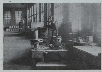
Crucible-forming Machine, showing mould and forming tool
