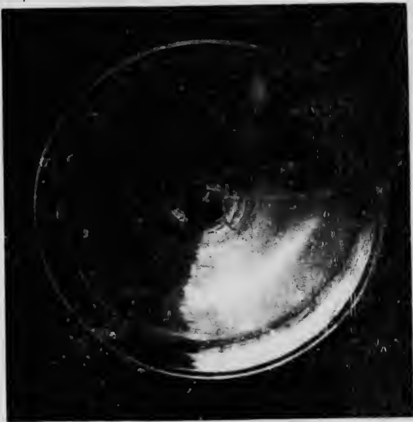
INTERIOR OF WINE-GLASS FOOT, SHOWING THE PONTIL-END AT THE CENTRE, AND THE FOLDED FOOT AT THE RIM.
