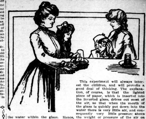
the water within the glass. Hence, the weight or pressure of the air on the water outside the glass drives the water up into the glass to occupy the space from whence the air was driven by the burning paper. A practical demonstration of this kind is always more convincing than
