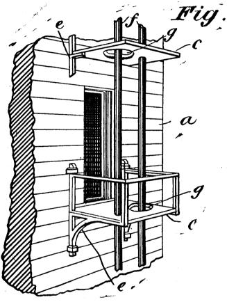
floors or staging from the root to the ground; g g are circular openings which alternate from one side to the other at each succeeding landing. The landing to be placed before a window at every story.
