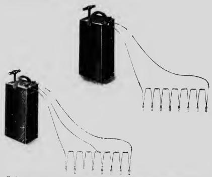
Series connection with blasting machine. The break in the wires is merely to indicate that any required length of wire may be used between electric fuzes and blasting machine. There must be no break in the actual circuit.
