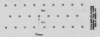
The entire cost, including labor and stumping of ditches from three to four feet deep, three feet wide at the bottom and five to seven feet wide at the top, is two cents to four cents per lineal foot or an average of about six and two-thirds cents per cubic yard excavated. Ditches requiring two or three rows of holes and those
