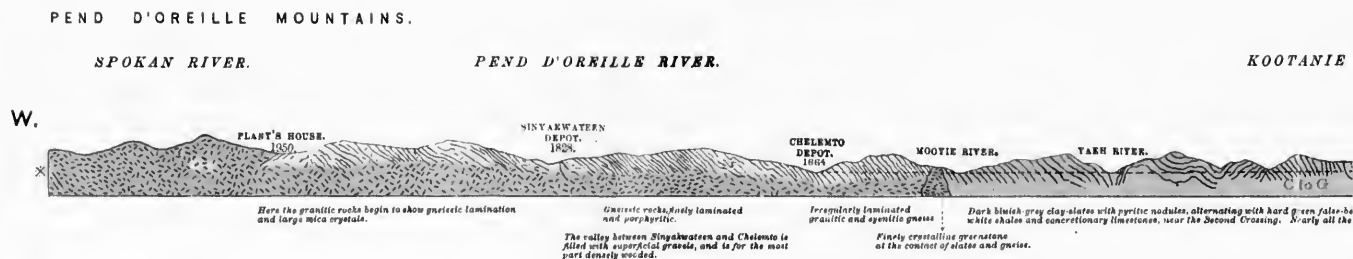
SECTION FROM FORT HOPE, FRASER RIVER, TO WATERTON, O. Constructed from observations made on the Brigade trails from Fort Hope to Colville, from Colville to the Kootanie Horizontal Scale, 10 miles to an Inch. Vertical Scale, 10,000 feet to an Inch. Heights in
