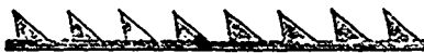
Garnett Wire. This wire is used for covering iron rollers, breasts of woolen cards, lickersin of cotton cards, comber doffers, etc.
