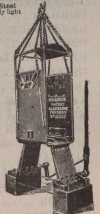
15—R. H.'s Improved Steel Cage, with Safety Grippers and Pullers complete
