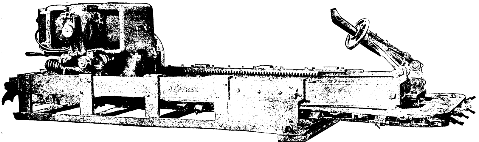
17A. Electric Chain Coal Mining Machine
