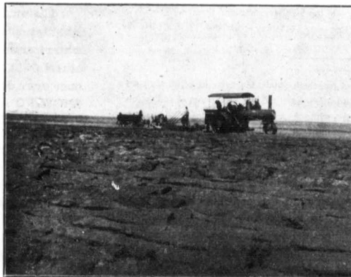
American-Abell 28 h.p. Steam Tractor Pulling an 8-bottom John Deere Engine Gang. (Winner Gold Medal, Class F.)
