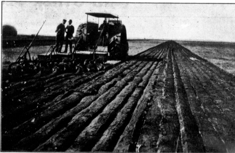
The "Flour City" Kerosene Tractor Performing the Plowing Feature of its Gold Medal Work. A John Deere 8-bottom Engine Gang is Being Pulled.
