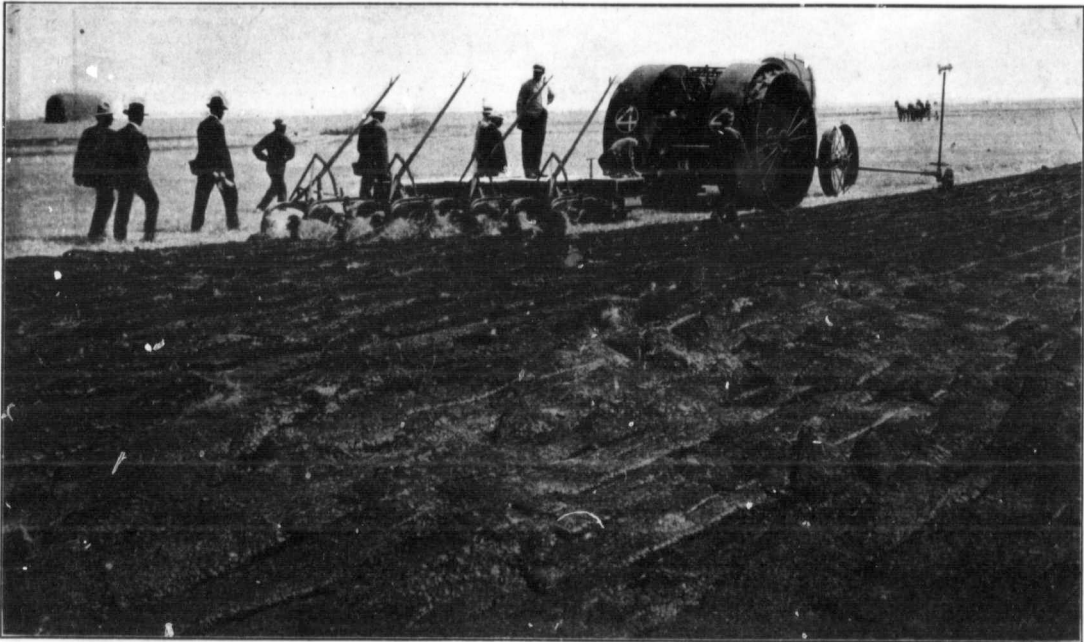
An eight-bottom 14 inch John Deere Engine Gang as pulled in the Motor Contest by the Gas Traction 30 (Winner of gold medal in Class C. Gasoline Engines).
