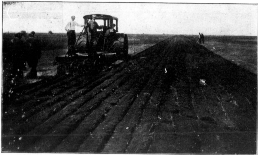
The American Abell Universal Farm Motor pulling a 4-bottom John Deere Engine Gang.
