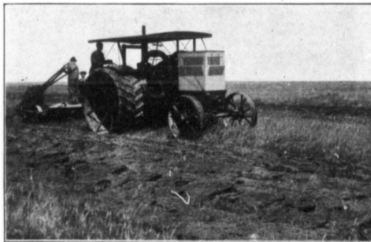
I.H.C. 25 H. P. Gasoline Engine pulling a P. and O. Plow (Winner of Silver Medal Class C)
