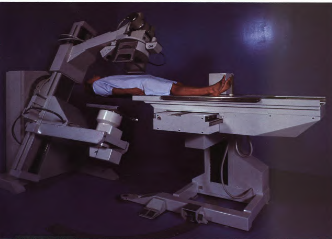
The Therasim 130, which simulates radiotherapy treatment.
