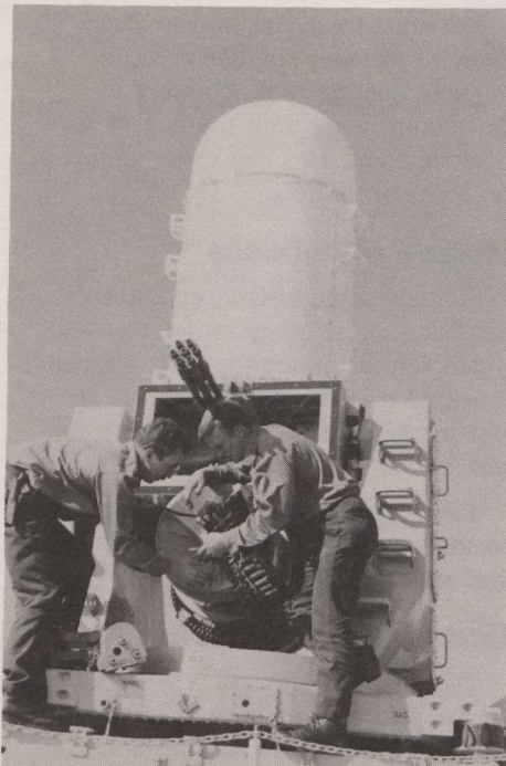
Canadian Forces personnel in the Persian Gulf fitting ammunition to the ship-board Phalanx air defence system. The Gulf War has made many countries take a closer look at controlling the arms trade.
