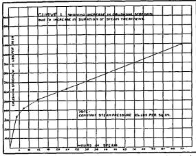
Diagram, Showing Increase in Crushing Strength, due to Increase in Duration of Steam Treatment.
