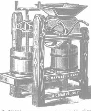
HOW many go to waste that might be turned into Cider or Cider Vinegar with a small investwell made, of the best material, heavy, substantial frame, and cross section of extra weight and strength; furnished with two crates, galvanized hoops and tinned rivets. Made for either hand or power.
