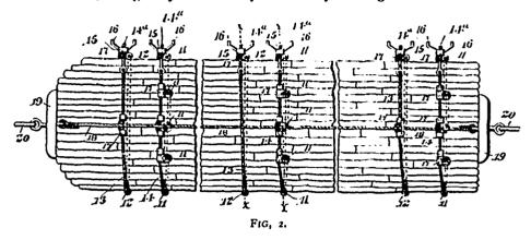
be employed, as desired. Each section is composed of timbers arranged end to end and having their joints disposed in staggered relation and therefore thoroughly broken. The sections extend from side to side of the raft, and each is tastened by separate binding-cables surrounding the same. Thus it will be apparent that each section is independent of the others, and should the upper one be removed the remainder will be intact. The several
