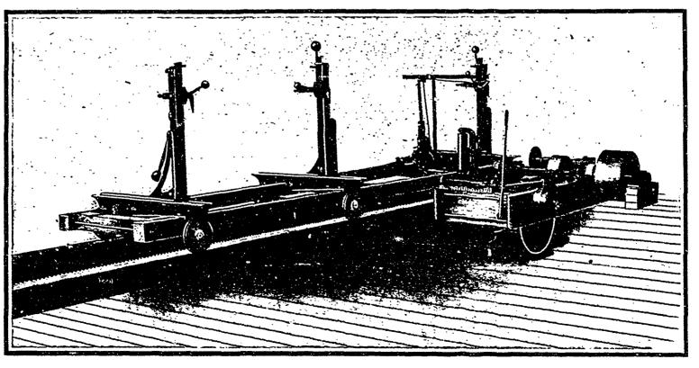
The above cut represents our new No. O Sawmill, Capacity 5,000 to 8,000 ft. per day, to carry up to a 56" saw.
