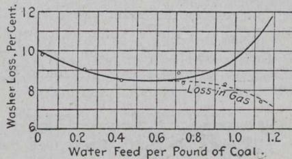
Fig. 6. Water Feed and Washer Loss.
