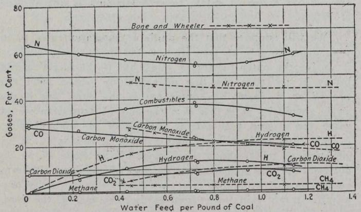
Fig. 1. Comparison of Present Tests with Those of Bone and Wheeler.
