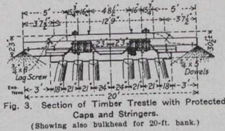
Fig. 3. Section of Timber Trestle with Protected Caps and Stringers. (Showing also bulkhead for 20-ft. bank.)
