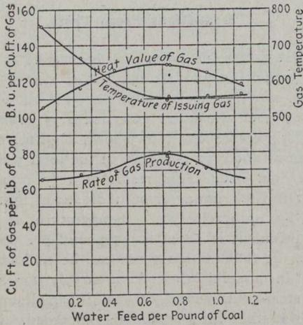
**Fig. 4. Effect of Water Feed Rate Upon Gas Made.**
