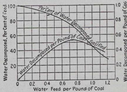
Fig. 2. Effect of Water Feed Rate Upon Decomposition.
