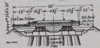
Fig. 5. Section of Ballasted Floor on Timber Trestle.
