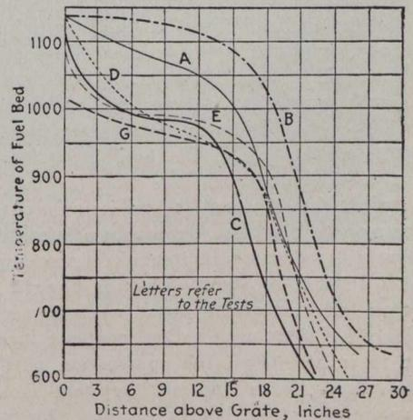
Fig. 3. Temperatures in the Fuel Bed.
