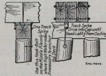
Fig. 2. Application of Casting Shown in Fig. 1. When it becomes necessary to line stringers, pull track spikes out of cap then shift stringers to desired position and redrive spikes through most favorable holes. Clean sand out of holes in castings thoroughly before driving spikes.
