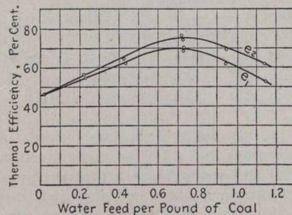
**Fig. 5. Water Feed and Heat Efficiency.**
