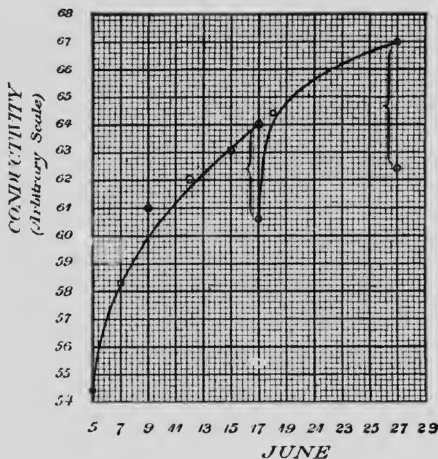
From these observations it would appear that the rise in the conductivity of the air in both cylinders may be divided into two parts and ascribed to different causes; the one being associated with some change in the surface of the metals used in the construction of the cylinders, and the other with some substance which becomes diffused throughout the air, and can be blown out with it.
