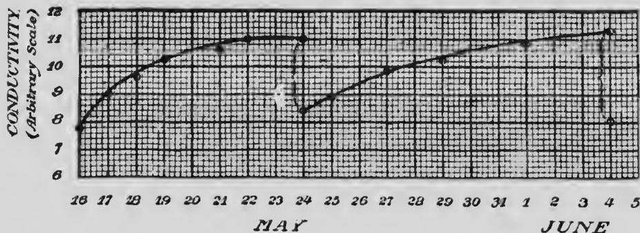
With cylinder No. 2 thoroughly cleaned in the manner already described, a reading of 54.5 divisions per minute with but slight variations was regularly obtained with freshly filtered air. With this cylinder, too, when the air was undisturbed in it the conductivity steadily rose, and after a time approached a maximum value. The time required for the steady state to be reached was, however, much greater than with cylinder No. 1.
