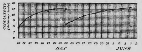
With cylinder No. 2 thoroughly cleaned in the manner already described, a reading of 54:5 divisions per minute with but slight variations was regularly obtained with freshly filtered air. With this cylinder, too, when the air was undisturbed in it the conductivity steadily rose, and after a time approached a maximum value. The time required for the st-ady state to be reached was, however, much greater than with cylinder No. 1.
