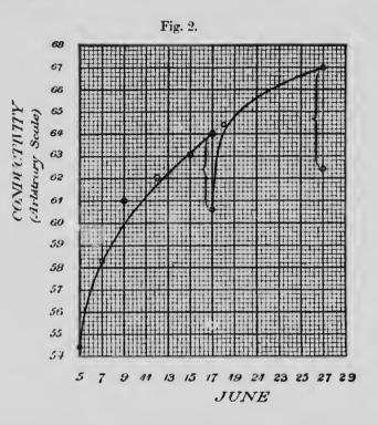
From these observations it would appear that the rise in the conductivity of the air in both cylinders may be divided into two parts and ascribed to different causes; the one being associated with some change in the surface of the metals used in the construction of the cylinders, and the other with some substance which becomes diffused throughout the air, and can be blown out with it.
