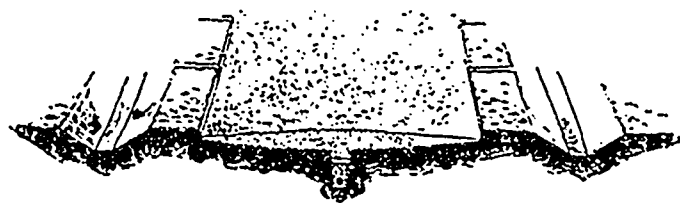
A gravel roadway with under-drain.
