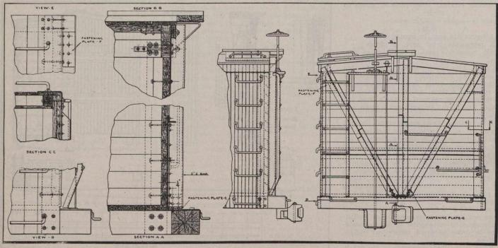
Fig. 3.—Reinforcement for New Cars.
