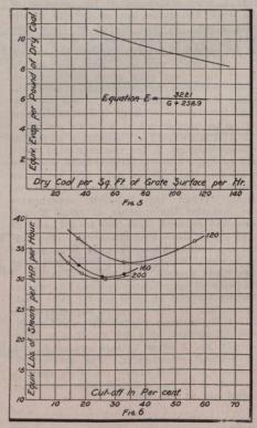
Fig. 5.—Relation Between Equivalent Evaporation per Pound of Dry Coal, and Dry Coal per sq. ft. of Grate Surface per Hour for Superheated Steam Locomotive.
