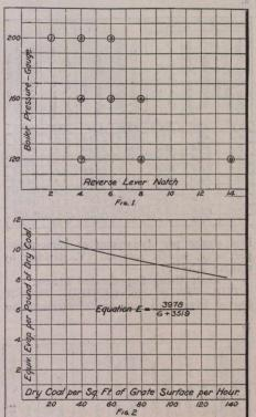
Fig. 1.—Conditions of Pressure and Cutoff for Saturated Steam Locomotive.
