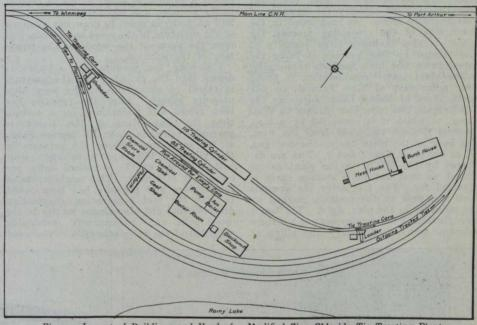
Fig. 1.-Layout of Buildings and Yard of a Modified Zinc Chloride Tie Treating Plant.
