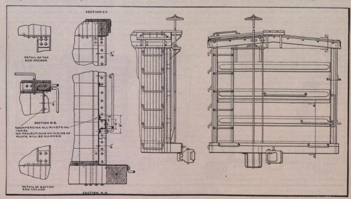
Fig. 2.—Reinforcement of Wooden Cars to Replace Broken Ends.
