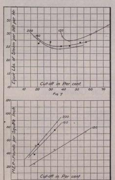
7.—Relation Between Equivalent Pounds of Steam per i.h.p. Hour and Cutoff for Superheated Steam Locomotive. 8.—Relation Between m.e.p. and Cutoff for Saturated Steam Locomotive.
