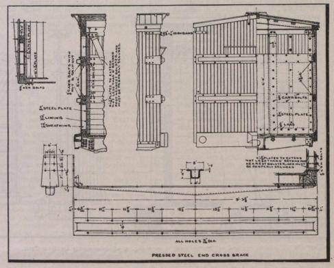
Fig. 1.—Reinforcement for Wooden Cars with Standard M.C.B. Lining.
