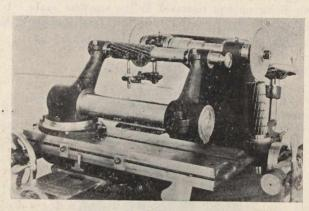
Fig. 4. Grinding Side and End of Taper Shank End and Side Mill.
