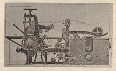
Fig. 32-Wet Machine, Waterous Engine Works Co.
