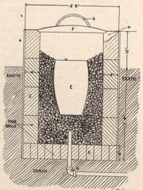
Fig. I.—An Emergency Brass Furnace.
