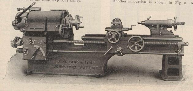
Fig. 1.—Twenty-inch Swing Triple-Geared Lathe.
