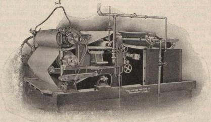
Fig. 33-Wet Machine (Jenckes Machine Co.).
