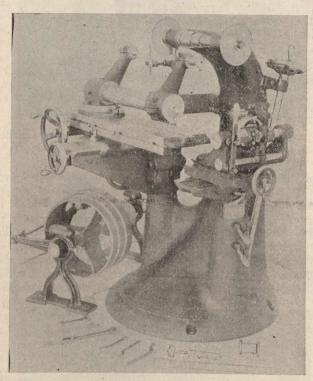
Fig. 1.—No. 1. Fourteen-inch Cutter and Reamer Grinder.
