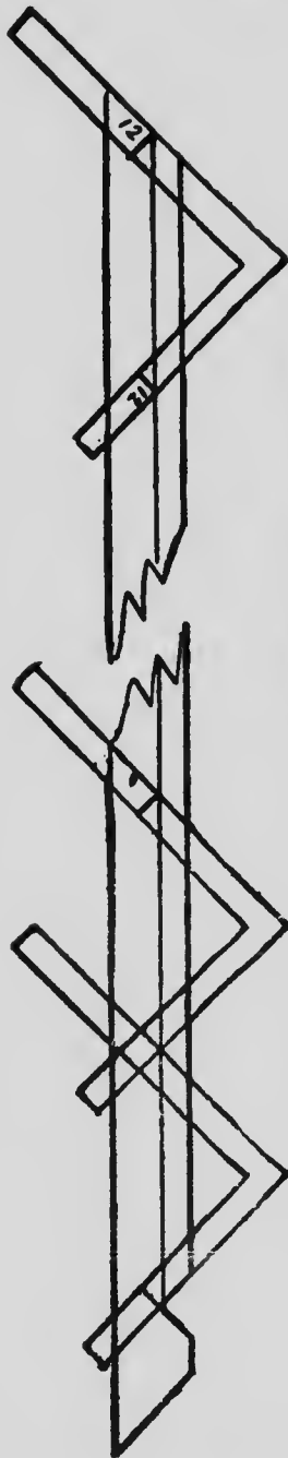
FIG. 36. SHOWING HOW TO LAY OFF A RAFTER WITHOUT MAKING USE OF A FENCE.
