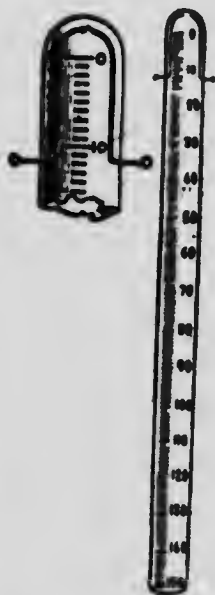
FIG. 14.—EUDIOMETER At the left is the upper end showing the platinum termin- als.
