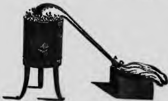
FIG. 34.—SCHEEL'S ORIGINAL DRAWING OF HIS METHOD OF PREPARING CHLORINE AND COLLECTING IT IN A BLADDER
