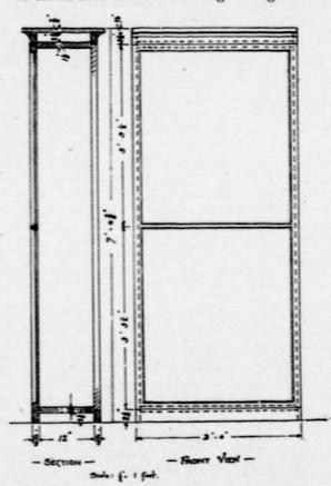
sary for supporting any shelves used. If a diaphragm is used, the screws to hold the rear corners of the shelves may be inserted in the diaphragm.
