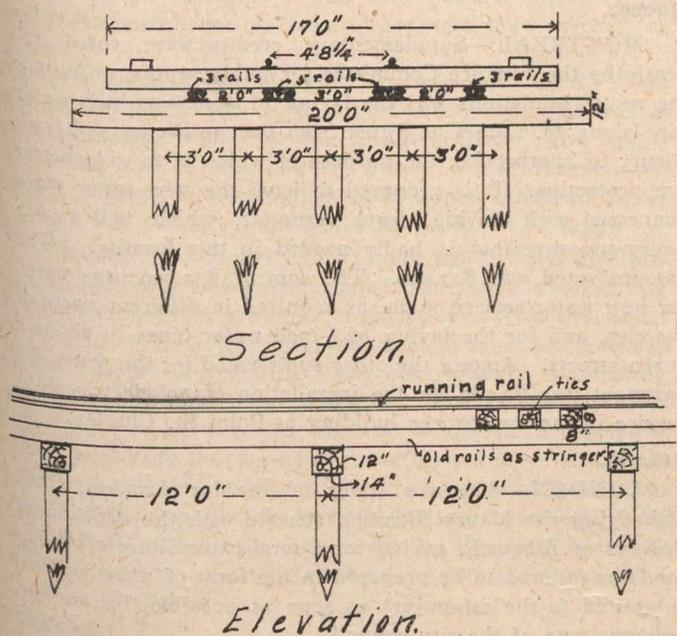
On this branch 65 pound rails were being replaced by 80 pound rails, and in renewing the bridges the old rails were used as stringers. Under the running rails a cluster of five 65 pound rails were used, and over the outside piles a cluster of three rails used. By means of spikes and 3/4-inch bolts through the fish plate bolt holes the rails are held in place. This bridge has carried for years the heaviest freight engines. Yours truly,
