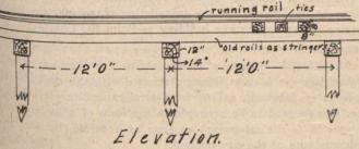
On this branch 65 pound rails were being replaced by 80 pound rails, and in renewing the bridges the old rails were used as stringers. Under the running rails a cluster of five 65 pound rails were used, and over the outside piles a cluster of three rails used. By means of spikes and 34-inch bolts through the fish plate bolt holes the rails are held in place. This bridge has carried for years the heaviest freight engines. Yours truly,
