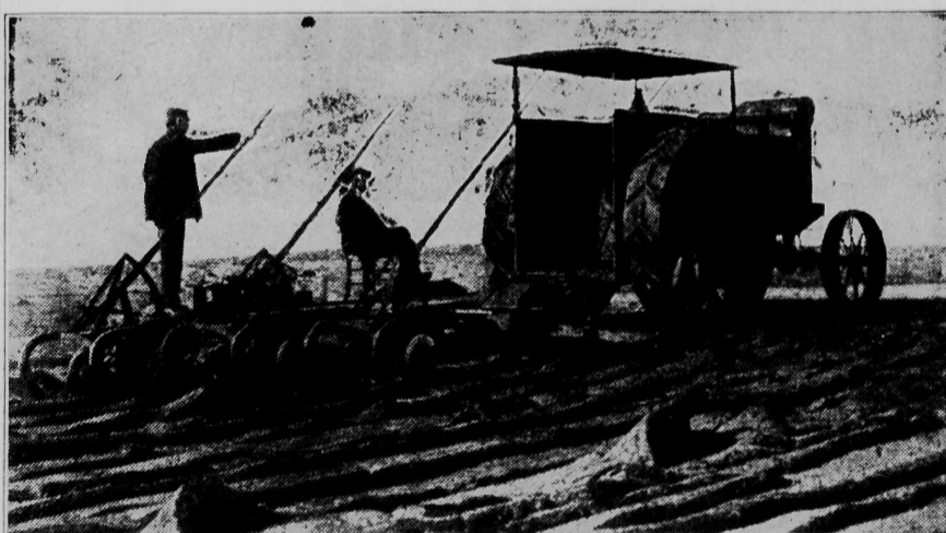
The 30 H. P. "Flour City" four cylinder Gasoline Engine pulling an engine gang of six plows in prairie sod.
