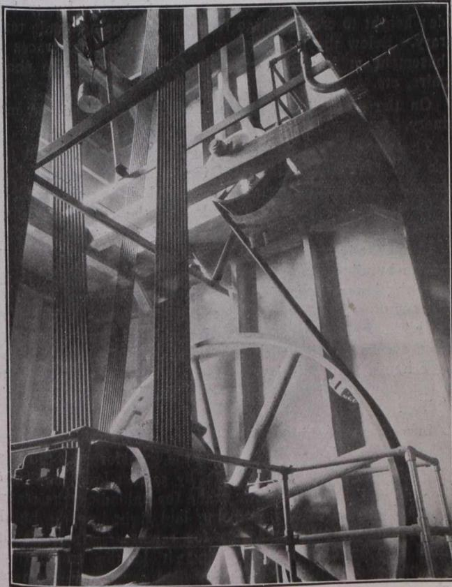
Fig. 8.—Drive to Receiving Elevator Leg.
