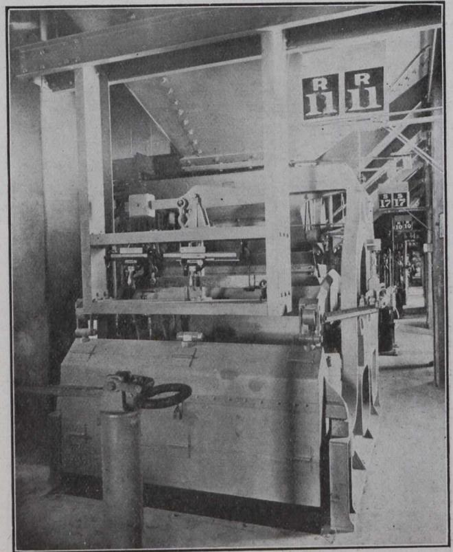
Fig. 7.—Automatic Weighing Machine, 5,000 lbs. per Draft.
