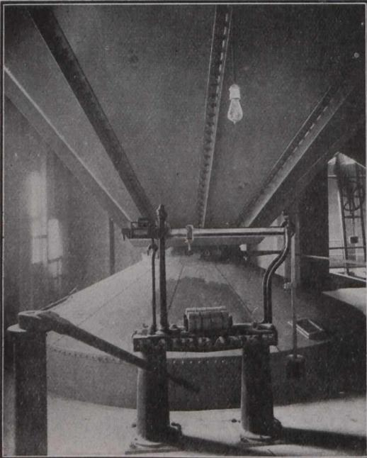
Fig. 6.—View of 2,000-Bushel Hopper Scale.
