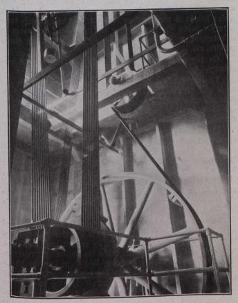
Fig. 8.—Drive to Receiving Elevator Leg.
