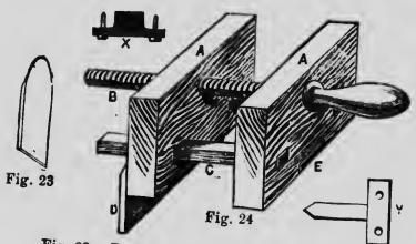
Fig. 23.—Plough Knife. Fig. 24.—Plougn.
