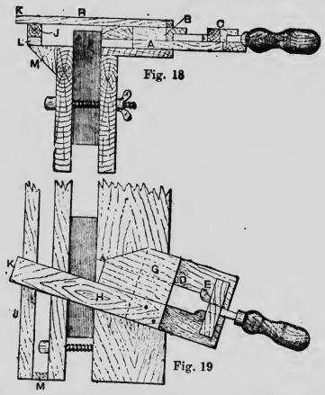
Fig. 18.—Elevation of Home-made Plough. Fig. 19.—Plan of Home-made Plough.
