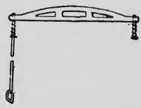
Fig. 27.—Clamp of Strawboard Cutter.
