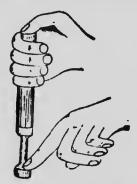
Fig. 104.-Method of Holding Lettering Tool.
