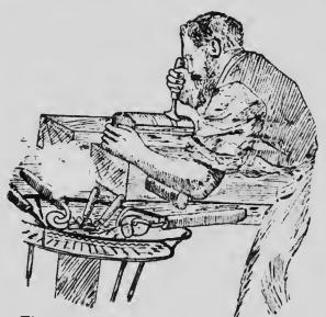
Fig. 105.—Method of Applying Pallet.
