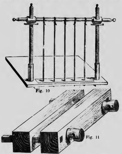
Fig. 10.—Sewing Press. Fig. 11.—Lying Press.
