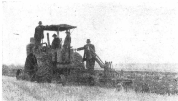
John E. Morin, Watson, Sask., using his "Rumely" with a six-bottom gang on stubble.
