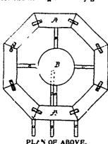
Part of a curtain pole, 12 inches long, serves as a splendid shaft, and curtain-pole sockets make an inexpensive and splendid bearing after they have been oiled a few times. The ship I borrowed from the toy department. I painted the scene with ordinary house paint on cotton. The blue skyline made a splendid contrast to the stone, and toned the color up fine. The display was a trade-winner, which was the object to be
