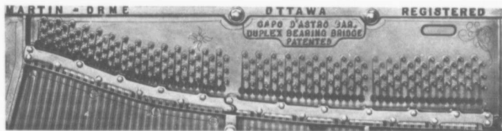
Newly Patented Martin-Orme Duplex Bearing Bridge and Capo D'Astro Bar
