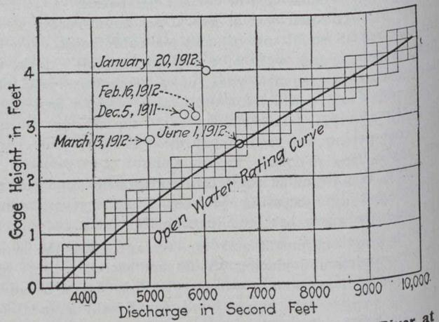
Fig. 1.—Open-Water Rating Curve for Rainy River at International Falls, Minn.
