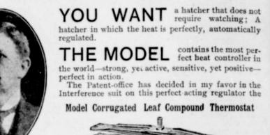
This Thermostat has three corrugations in each leaf, is exceedingly strong and frigid ; is not easily damaged ; and is so positive in action that the entire movement given off by the different co-efficient of expansion between the two metals of which it is made is transmitted to the controlling device without any loss of movement.
