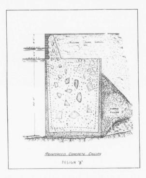
well off shore, and there would be considerable risk from leakage and sinking. The preparation of the bottom to receive the caissons would entail serious expense. In many places it would be necessary to dredge solid rock to depths ranging up to 20 feet and a full width of say 35 feet, in order to prepare a bed for the caissons.
