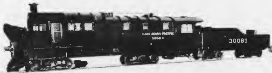
SIDE VIEW OF THE HUGE ROTARY SNOW-PLOUGH BUILT BY THE CANADIAN PACIFIC RAILWAY FOR SERVICE AMONG THE ROCKY MOUNTAINS
