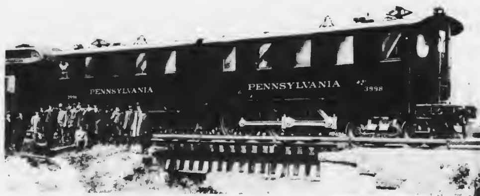
THE LARGEST AND MOST POWERFUL ELECTRIC LOCOMOTIVE IN THE WORLD It develops 4,000-horse-power and is employed for hauling trains through the New York tubes of the Pennsylvania Railroad Company.
