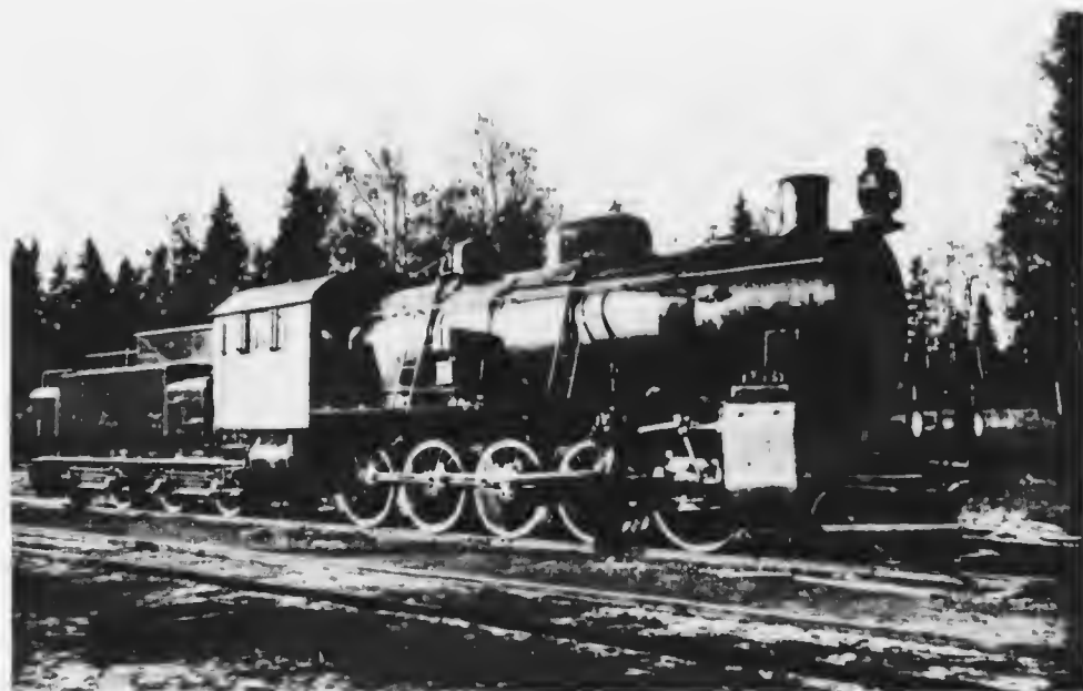
HEAVY TEN-WHEELED COUPLED LOCOMOTIVE USED IN THE IRON ORE TRAFFIC OF SWEDEN. The engine weighs 83½ tons, the whole of which is available for adhesion.
