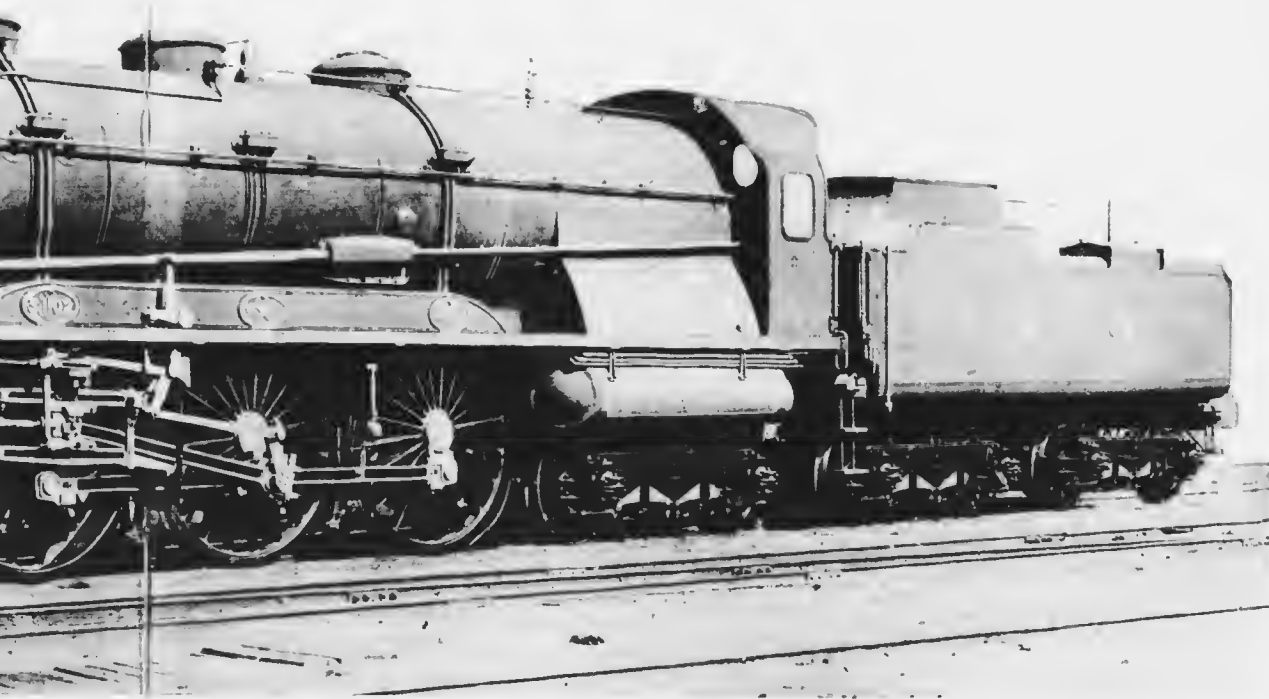
LOCOMOTIVE OF THE CHEMIN DE FER DU NORD. a train weighing 400 tons at 75 miles per hour on the level, and at 60 miles per hour up grades of 1 in 200.
