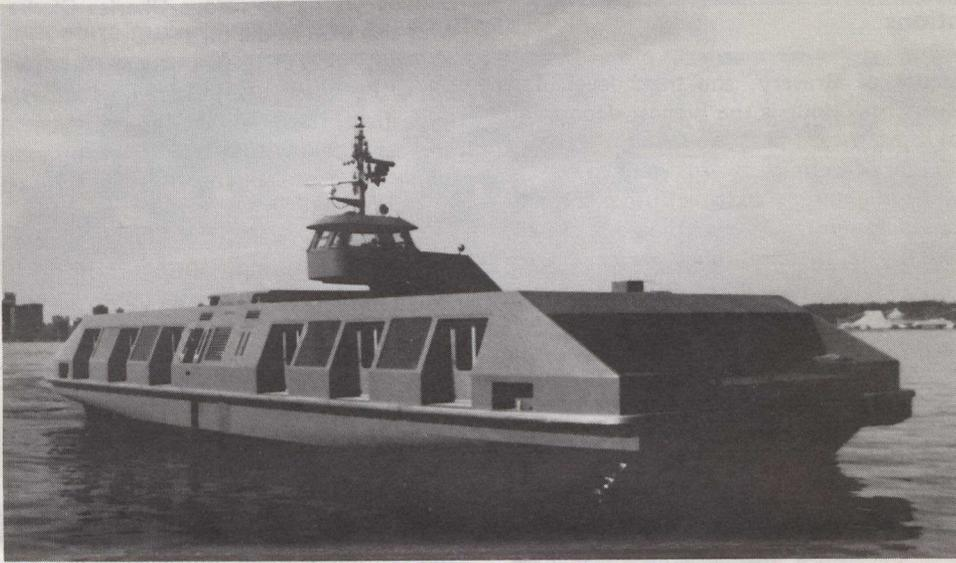
The 12-minute ferry link between downtown and North Vancouver is one element in a master design that also includes passenger terminals and city buses. Seabus, which carries 8 000-12 000 passengers daily, was designed by Case Existological Limited.
