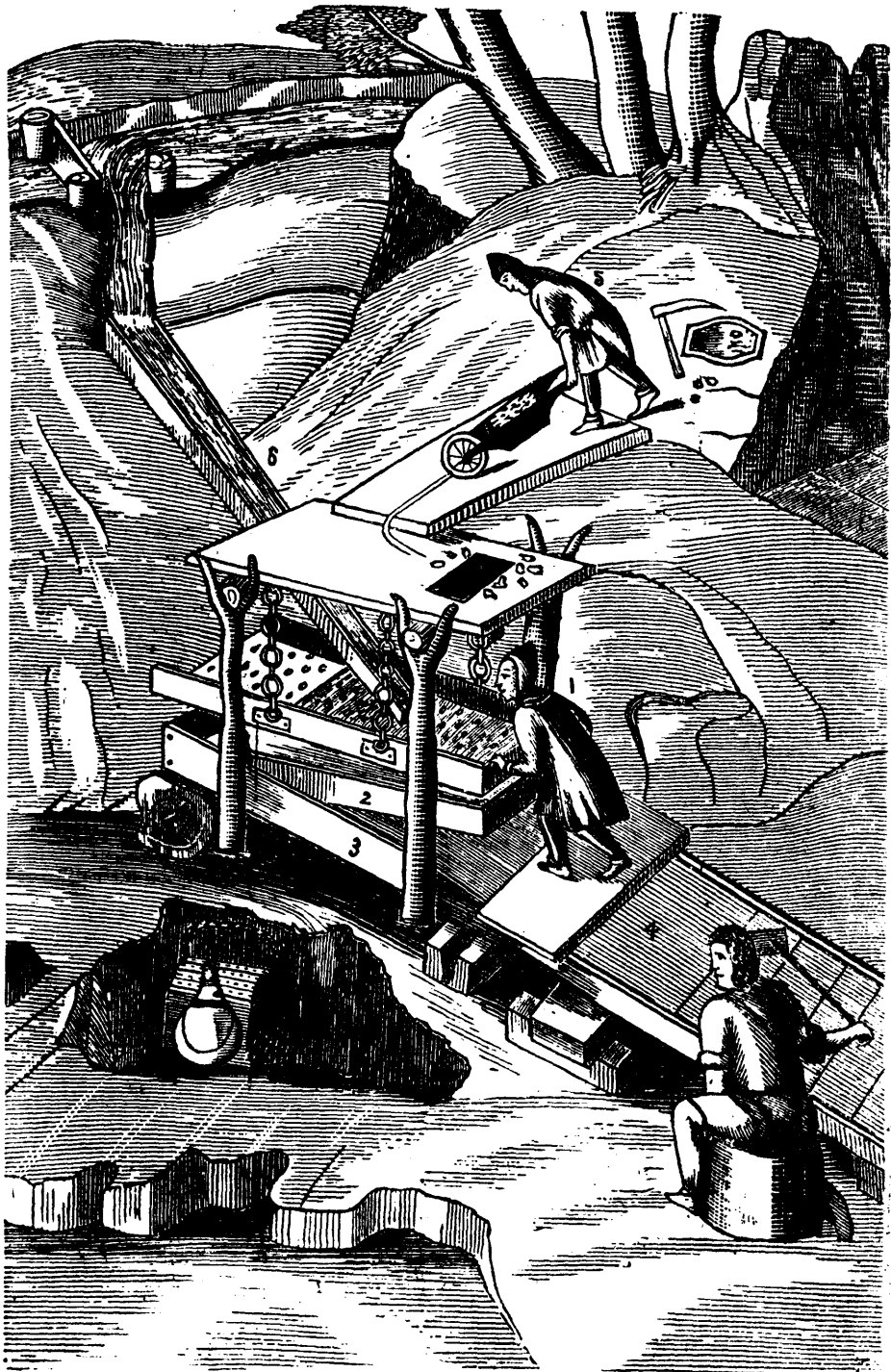
FIG. 1.—MACHINE FOR WASHING GOLD ALLUVIA 200 YEARS AGO. THE MINING OF GOLD QUARTZ.
