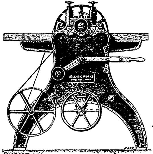
FIG. 2. ROLLER-FEEDING PLANING MACHINE
