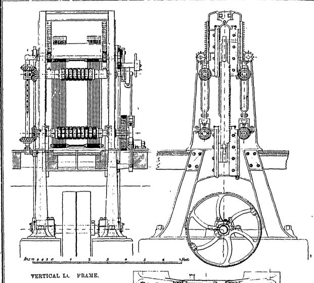
We illustrate, on this, and the opposite page, a saw frame for cutting logs, which may be taken as the type of these machines as made by the leading manufacturers in Austria and Germany, and of which many examples were found in the Machinery Hall of the Vienna Exhibition, although Messrs. Wannieck & Co., of Brunn, the makers of the machine we illustrate, did not exhibit one.
