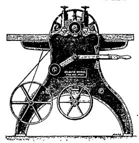
Fig. 2. RGLLER-FEEDING PLANING MACHINE
