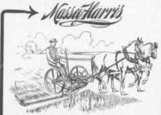
T has ample power for cutting the heaviest hay. Cutter bar is free to follow uneven ground. Lift Spring may be adjusted to carry as much or as little of the weight of cutter bar as conditions require. Raised Ledger Plates give extra long cutter edges and the edges are serrated. Cutter Bar has great range of tilt. No "flying start" required-the knife begins to cut the instant horses start. The easily operated foot lift enables the driver to quickly raise the bar for passing obstructions.
