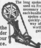
The long spokes of the Eccentric Sprocket used on Frost & Wood Binders give the necessary power to compress and tie each bundle thoroughly, then the short spokes make the discharge arms act quickly and get that sheaf out of the way of the next. This feature is worth any man's while to investigate. It and numerous other distinctive advantages of this machine are described in our Binder Booklet. It will pay you to get posted.
