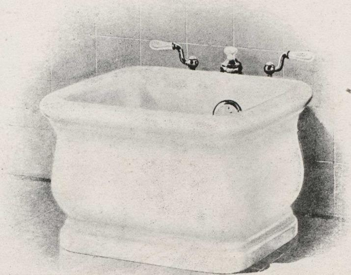
"ALEXANDRA" WARE—PLATE F. 035.—FIRST GRADE ENAMELLED OUTSIDE AND INSIDE *FOOT BATH* ON BASE. NICKLE-PLATED FULLER BELL SUPPLY AND WASTE FITTING, CHINA HANDLES AND CHINA WASTE KNOB. *DIMENSIONS*—LENGTH OVER ALL, 22 INCHES; WIDTH OVER ALL, 19 INCHES; WIDTH OF ROLL RIM, 2 1-4 INCHES; DEPTH INSIDE, 11 INCHES.
