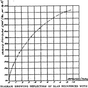
DIAGRAM SHOWING DEFLECTION OF SLAR REINFORCED WIT TRIANGULAR MESH.
