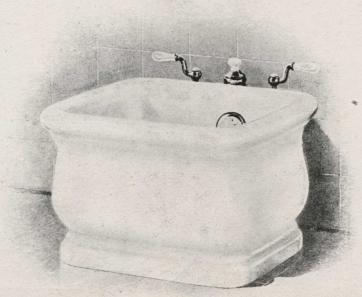
"ALEXANDRA" WARE—PLATE F. 035.—FIRST GRADE ENAMELLED OUTSIDE AND INSIDE FOOT BATH ON BASE. NICKLE-PLATED FULLER BELL SUPPLY AND WASTE FITTING, CHINA HANDLES AND CHINA WASTE KNOB. DIMENSIONS—LENGTH OVER ALL, 22 INCHES; WIDTH OVER ALL, 19 INCHES; WIDTH OF ROLL RIM, 2 1-4 INCHES; DEPTH INSIDE, 11 INCHES.
