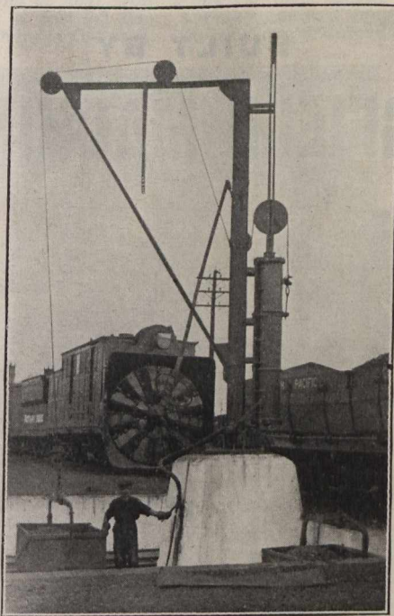
Fig. 2.—Radial Air Hoist for Raising Loaded Ash Cars.
