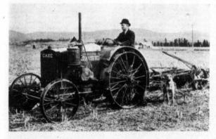
The tractor is equipped with some of the latest features in conveniences. There is a new air washer, especially needed in tractors, since they pick up so much dust in farm work, and the gears are enclosed making them dustproof. The engine is the fourcylinder type, valve-in-head, made in the Case factory. The tractor runs with either distillate or kero-The tractor is one of the lighter types, weighing when ready for the field 3,600 pounds.
